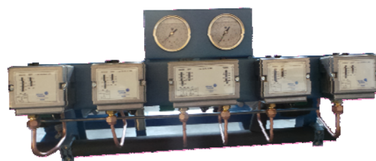
Alarm and control pressure switches
